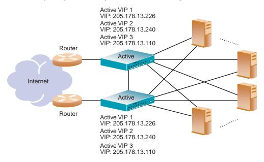
Figure 11-5 Active-Active Redundancy
